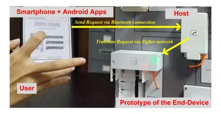
Figure 12. Setup for functional test result of curtain device
