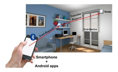
Figure 3. Architecture of the curtain control system
